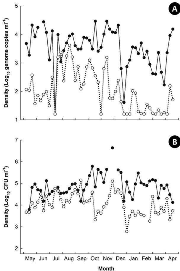
**Fig. 2.** Quantitation of viable *A. butzleri* DNA (A) and fecal coliform indicators (B) in untreated wastewater at the Lethbridge (solid lines) and Fort Macleod (dotted lines) WWTPs from May 2008 to April 2009. In Figure 2A, values presented as  $1.2 \log_{10}$  genome copies  $\text{ml}^{-1}$  represent results below the limit of quantitation for *A. butzleri* DNA.
