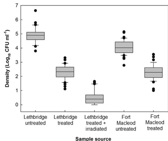
**Fig. 4.** Quantitation of fecal coliform indicators in wastewaters from the Lethbridge WWTP (A) and the Fort Macleod WWTP (B) from May 2008 to April 2009. A total of 52 samples were processed per sample source. Samples were collected at each WWTP immediately prior to treatment (untreated), and after mechanical/biological treatment (treated), and also at Lethbridge after UVB irradiation (treated + irradiated).
