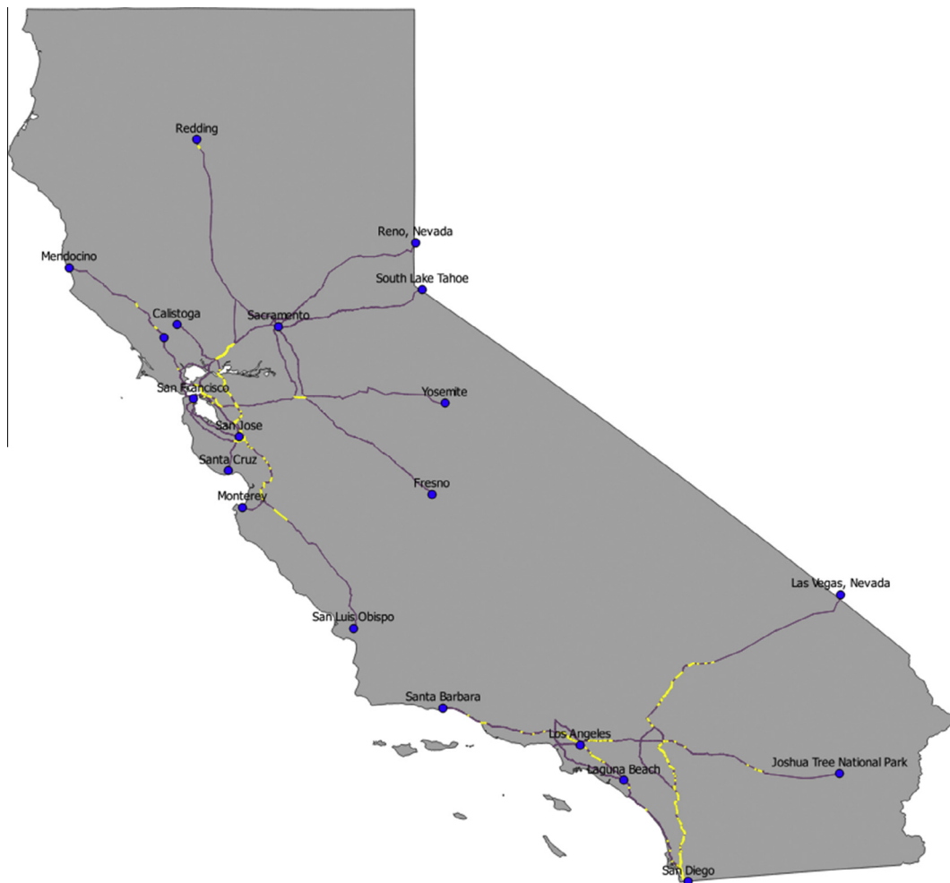
Fig. 2. 100 kW dynamic wireless charging infrastructure layout (wireless charging segments are highlighted in yellow). (For interpretation of the references to color in this figure legend, the reader is referred to the web version of this article.)
