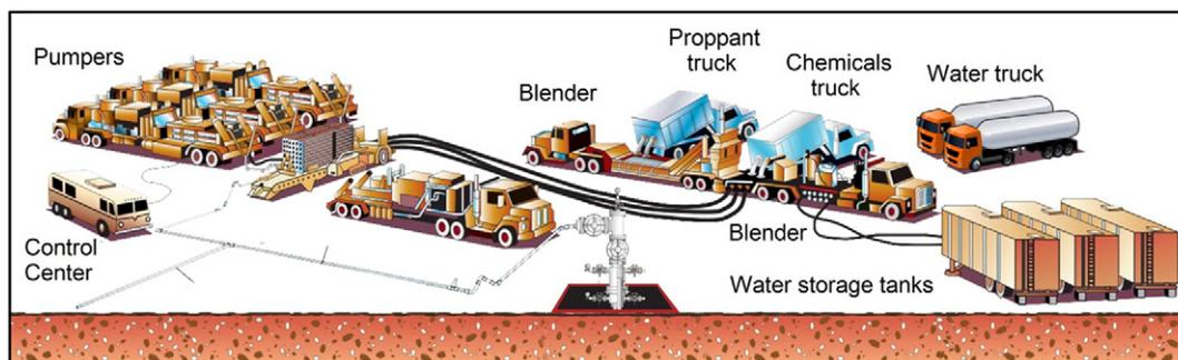
**Fig. 3.** Hydraulic fracturing units.
