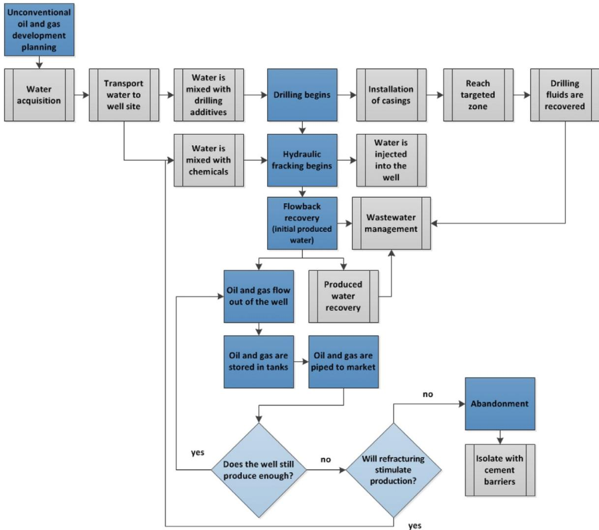
Fig. 2. General process of unconventional oil and gas production.
