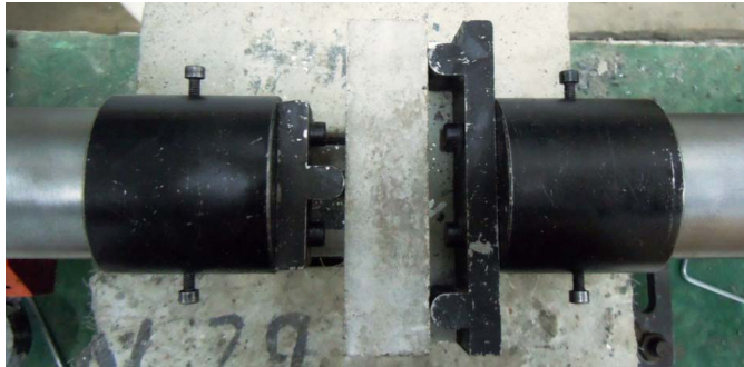
Fig. 2. Loading device of dynamic three-point bending test
