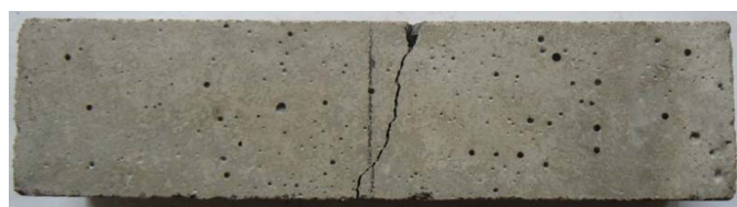
Fig. 4. Typical fracture pattern of concrete specimen
