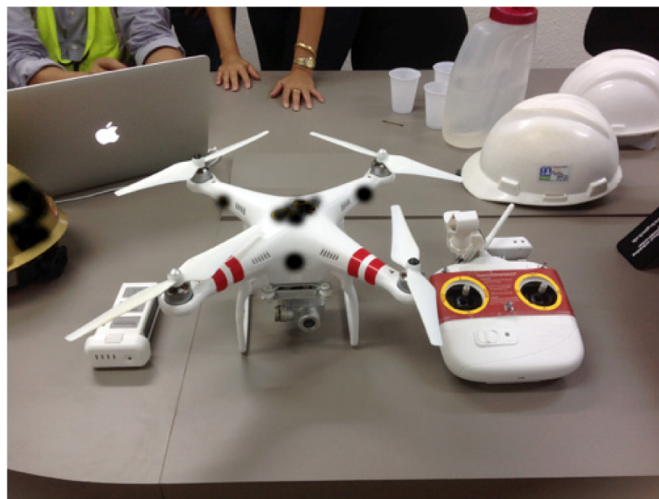
Fig. 3. DJI phantom 2Vision + UAS used in study (image by Javier Irizarry)
