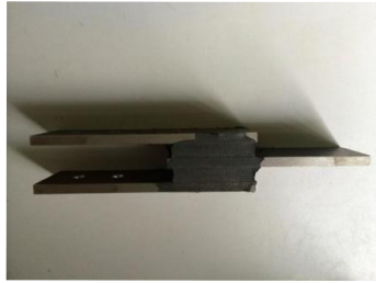
Fig. 1. Structure of a VE damper
