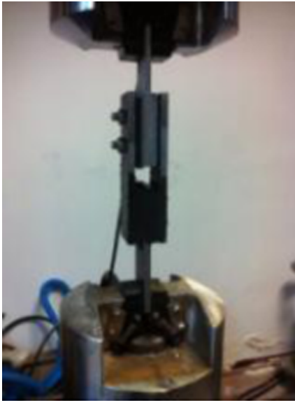
Fig. 2. Test loading device
