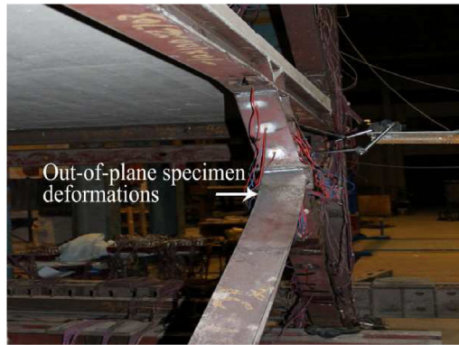
(f) Plastic hinge on the first storey
