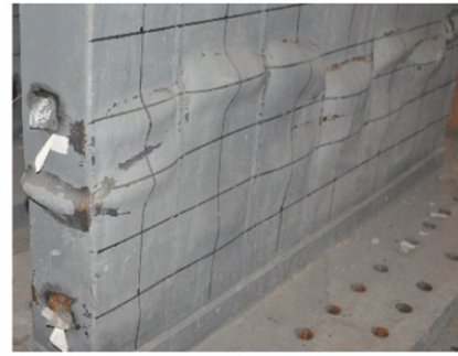
(a) Local buckling from the side view
