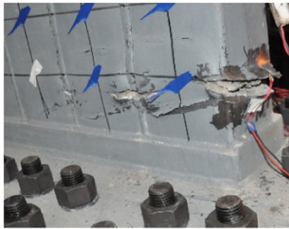
(b) Fracture propagation
