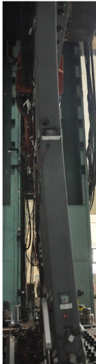
(c) Out-of-plane deformation
