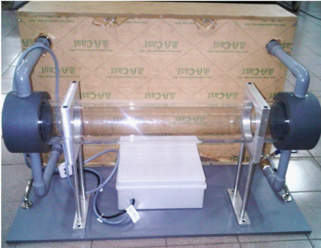
Fig. 10. Horizontal water/oil flow rigs.
