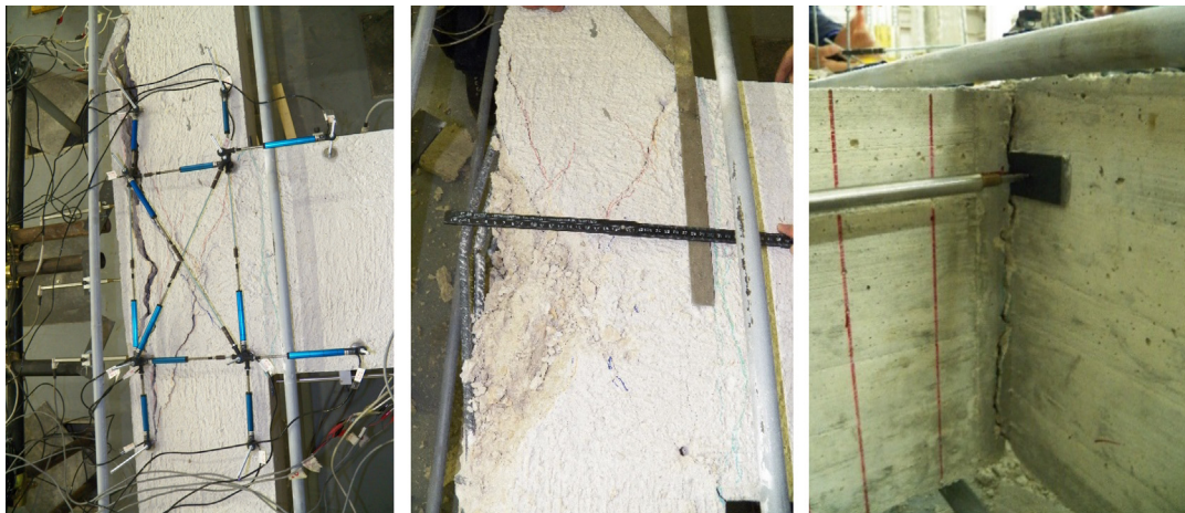
Fig. 11. Final damage state: joint panel and beam–joint interface – Test #2.
