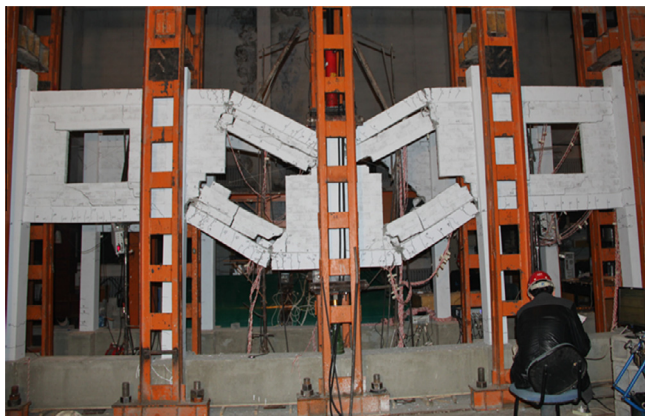
Fig. 12. Failure mode of the infilled frame at the end of the test.
