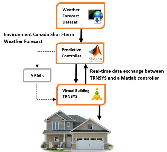
Fig. 3. Framework of the house energy simulation system.
