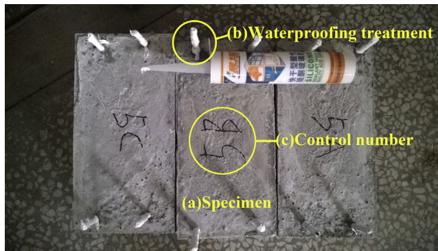
Fig. 2. Waterproofing treatment of steel bar.
