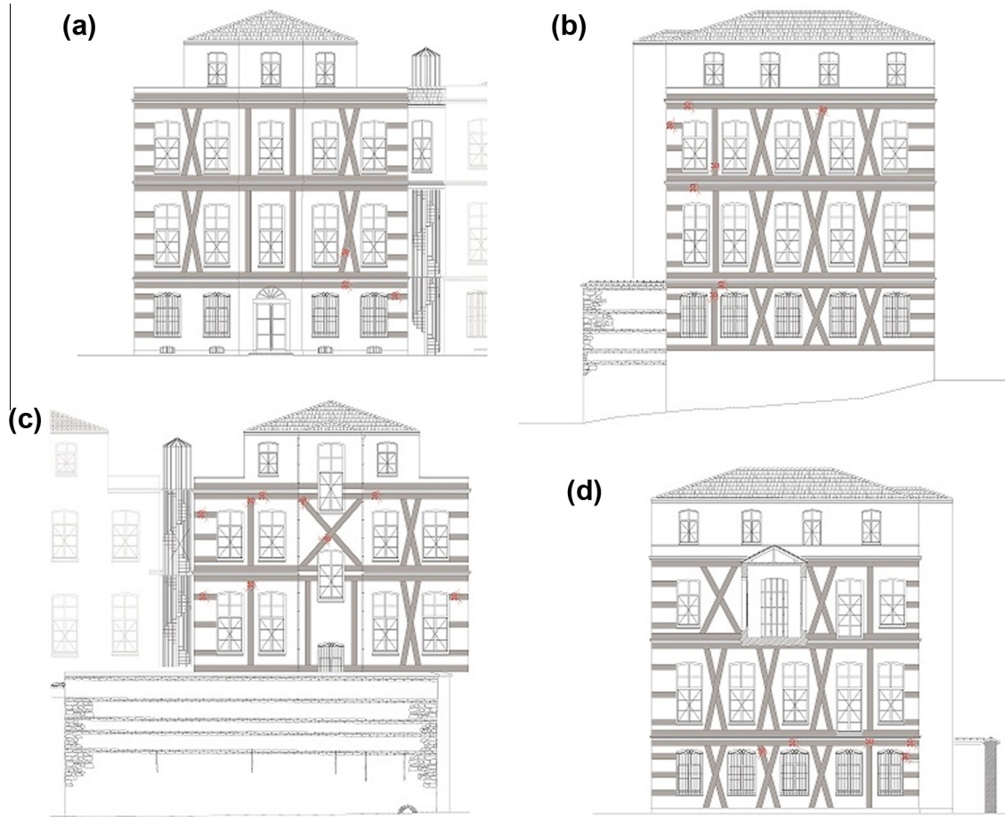
Fig. 10. Location of carbon fiber wrap application on four facades: (a) Southern facade, (b) Western facade, (c) Northern facade, (d) Eastern facade.
