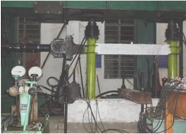
Fig. 26. RACFST plane frame: test setup (Chen et al. [68]).
