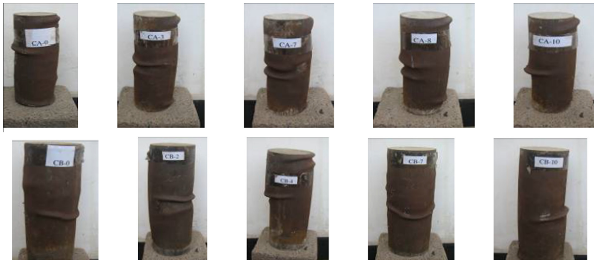
Fig. 13. Failure patterns of specimens (Chen et al. [34]).
