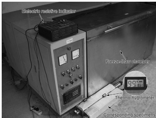
Fig. 5. Freeze-thaw test apparatus and control group specimens A-b-U and A-u-U monitored in real time by the thermo-hygrometer.
