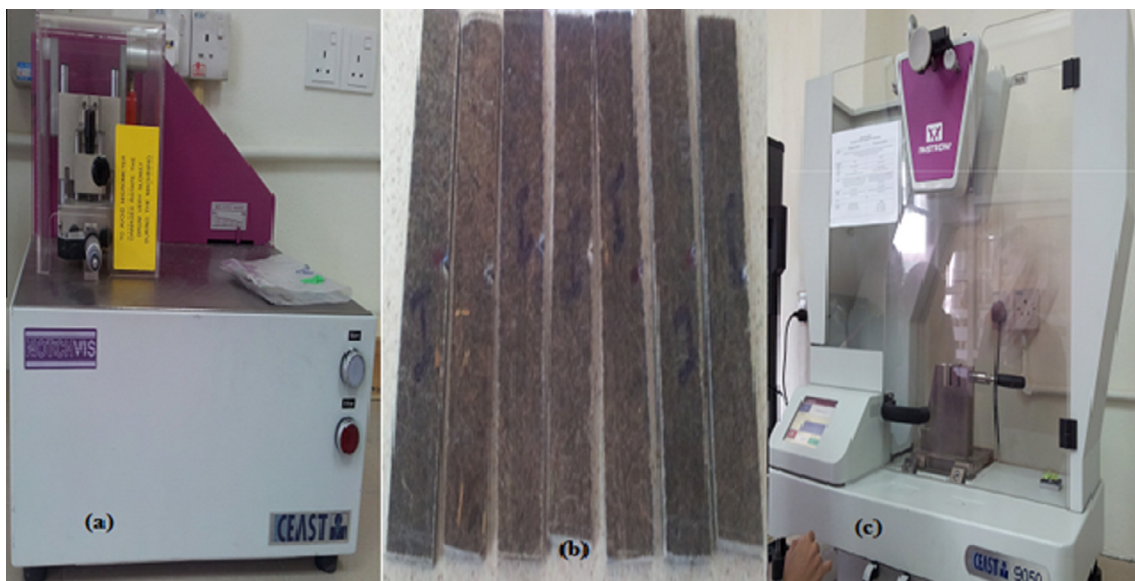
Fig. 3. (a) V-notched making machine (b) 7-V-notched specimens and (c) Impact testing instrument (INTROP).
