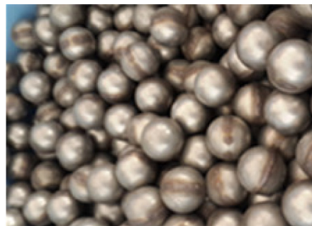
(b) Hollow sealed thin-wall steel balls
