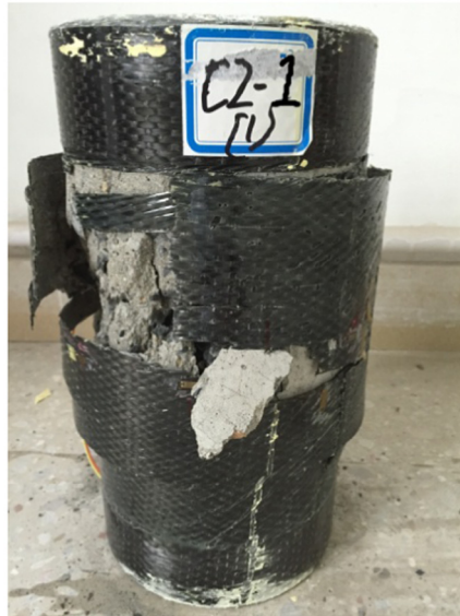
(b) CFRP-confined ceramsite concrete column
