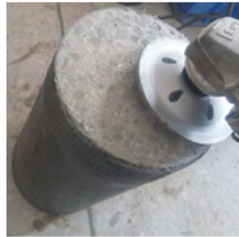
(b) End leveling of the ceramsite concrete
