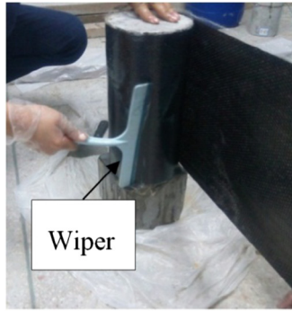
(a) Wrapping of the LWAC columns with the CFRP sheets
