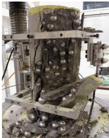
(a) Plain steel ball concrete columns
