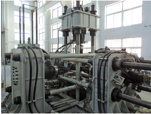
Fig. 1. Photo of the electro-hydraulic servo multiaxial testing system.
