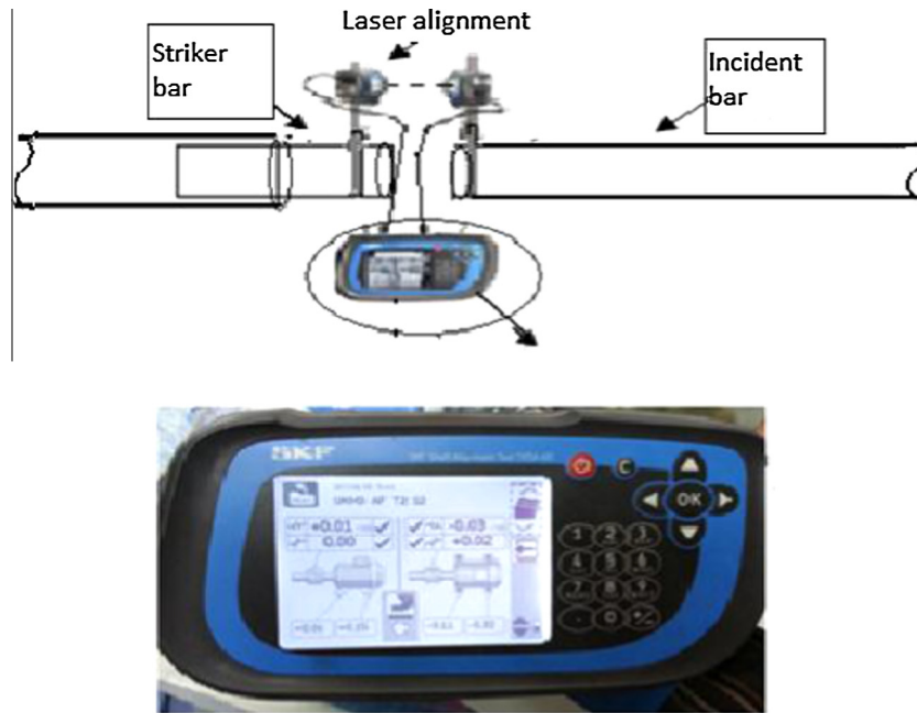
Fig. 3b. Laser alignment of the bars.
