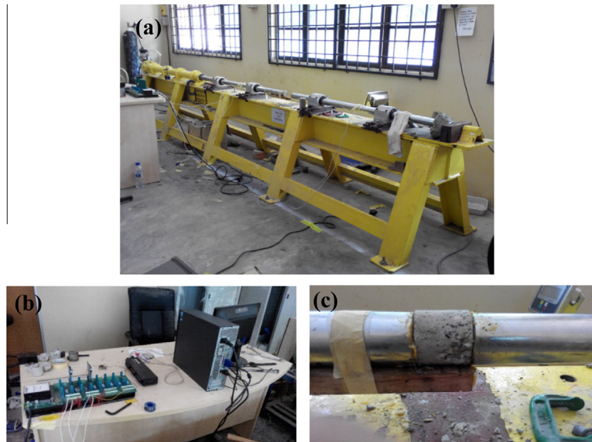
Fig. 2. View of the SHPB system: (a) SHPB equipment; (b) signal conditioner with oscilloscope connected to a computer and (c) concrete specimen between incident bar and transmission bar.
