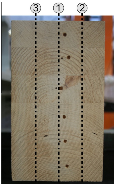
Fig. 8. Cross-section of the tested beam made from glued laminated timber with axes marking out the points where drilling resistance measures were taken (the openings visible result from tests carried out with stress wave and ultrasonic techniques).
