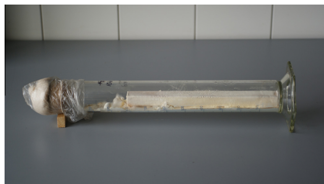
Fig. 1. Set up of the decay tests with wood samples on malt agar media.
