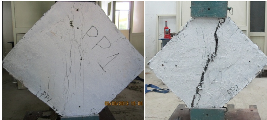
Fig. 8. Polypropylene jacketed walls: (a) cracks developing; (b) major crack and failure of second specimen.
