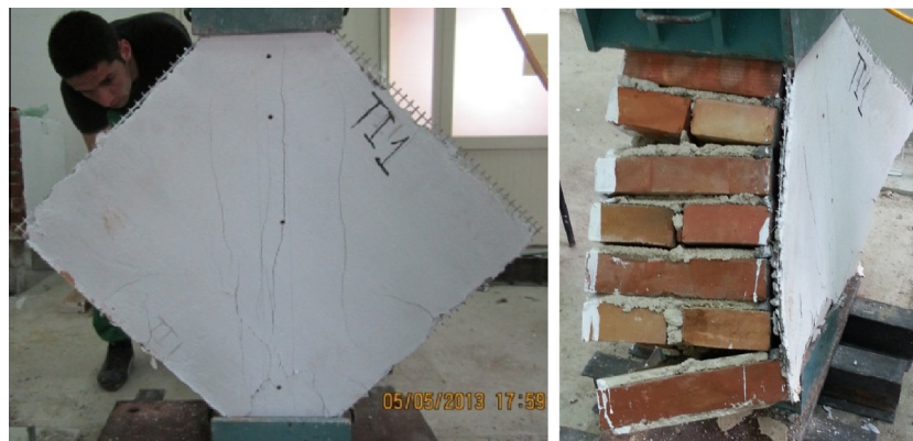
Fig. 6. TRM jacketed walls on one side only (TI): (a) crack development on the strengthened side, (b) inward bending of the strengthened side while cracks are still minor.
