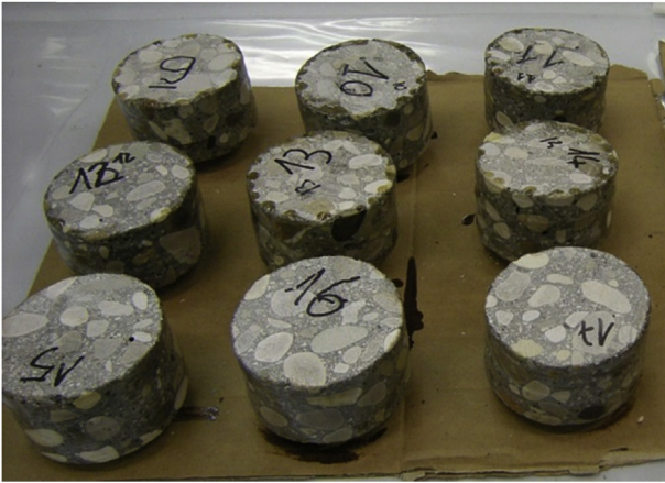
Fig. 3. Concrete cylinders used for chloride-ion penetration tests.
