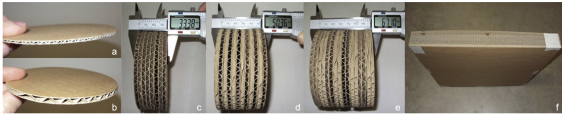
Fig. 1. Images of the considered samples: (a) E-flute; (b) C-flute; (c, d, e, f) parallel, orthogonal 1 × 1 and 2 × 2, and sandwich (4E-10C-4E) samples.
