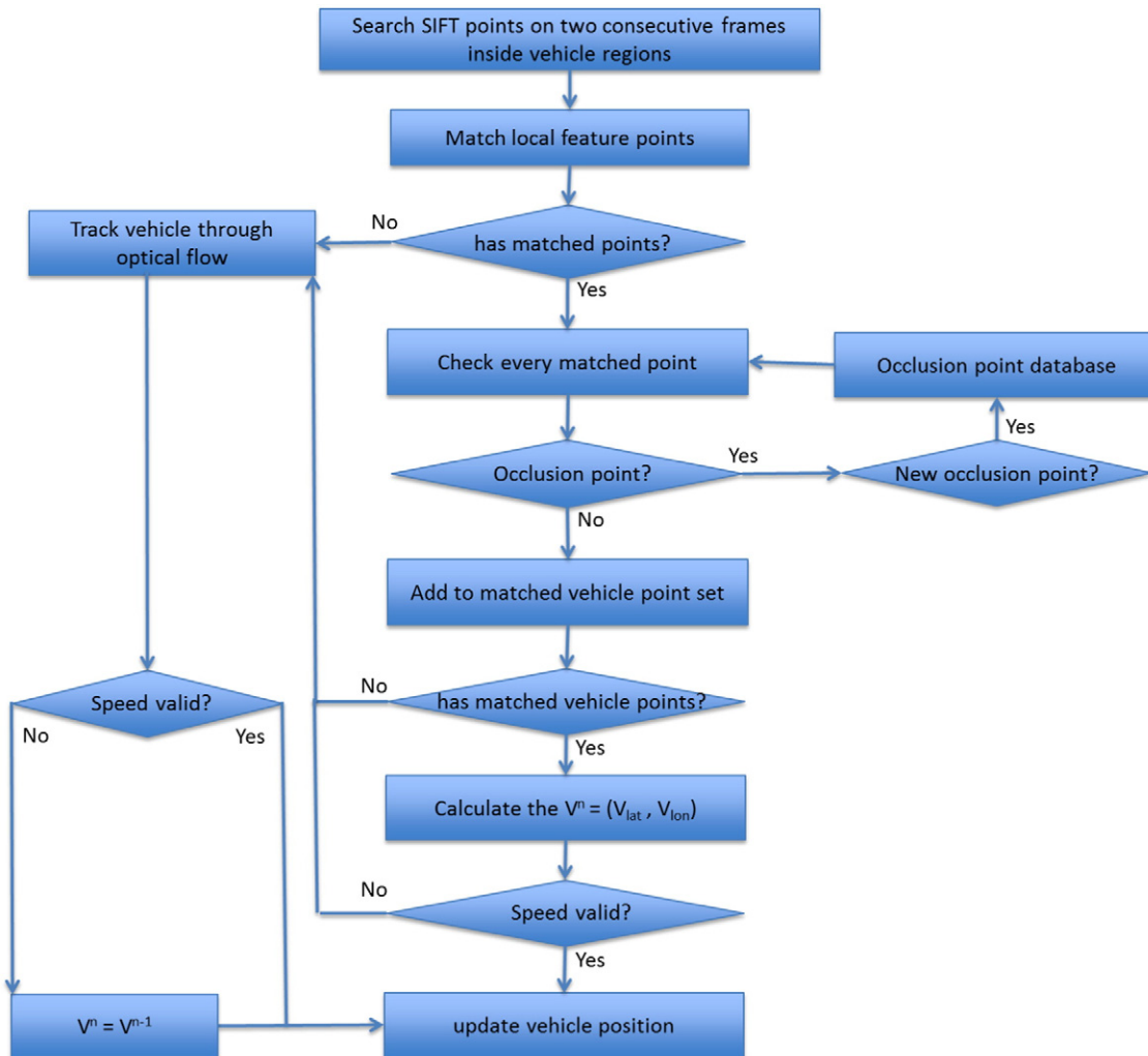
Fig. 12. Workflow of vehicle tracking.
