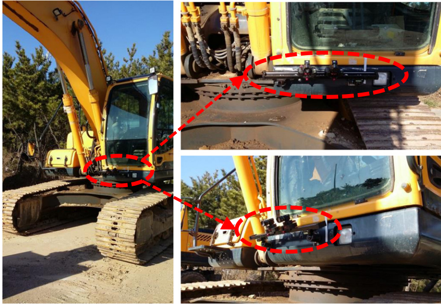
Fig. 12. Stereo camera system mounted on an excavator.
