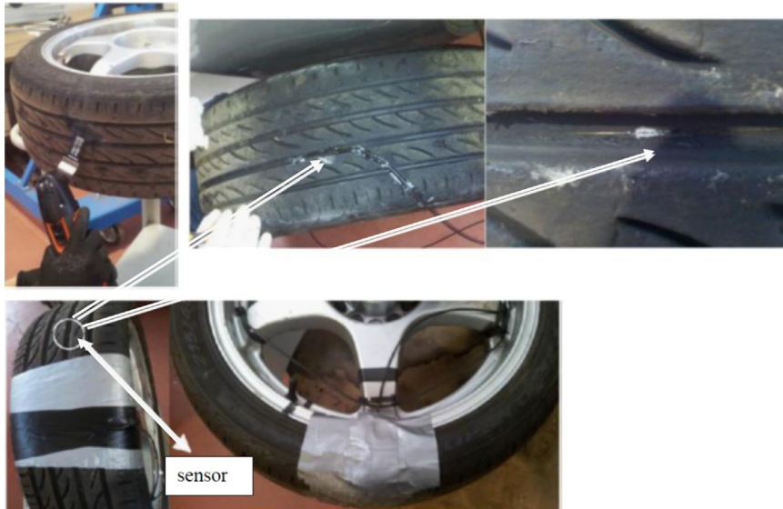
Fig. 3. Optical fiber pasted into the central groove of the tire tread. Preparation of the tire for the placement along the external circumference, the scotch tape protects the FBG sensors from the contact with the ground.
