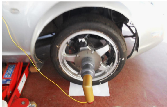
Fig. 16. Static measurements of the tire footprint.
