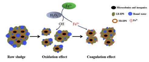
Fig. 7. Fenton oxidation and Fe(III) coagulation two-step mechanism of Fenton conditioning of sewage sludge.
