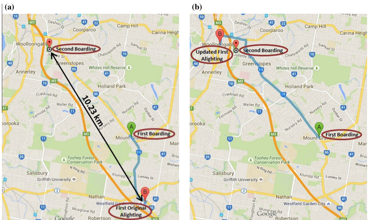
Fig. 1. Example of smart card transactions with a wrong alighting stop. (a) Wrong transactions and (b) potentially actual transactions.
