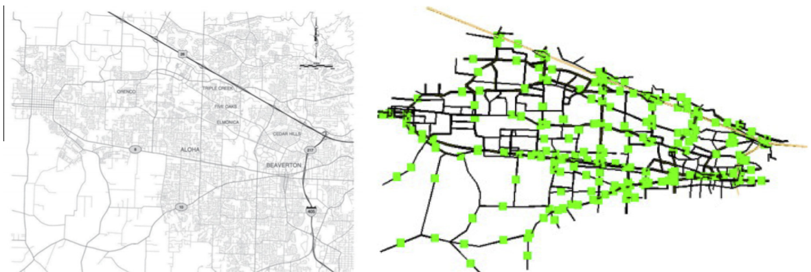
Fig. 11. Portland Beaverton subarea network adapted from SHRP II C05 project, rectangles on the right represent sensor locations for demand calibration.
