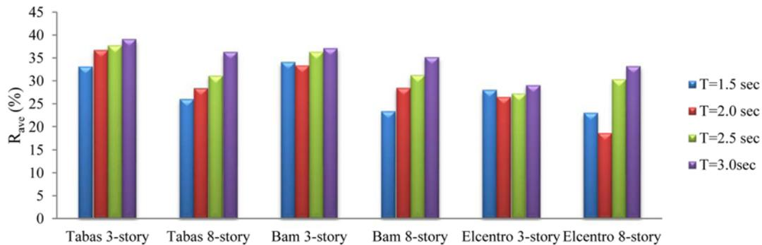
Fig. 13. Average Reduction of Torsional Responses of Model D in Comparison with Model A
