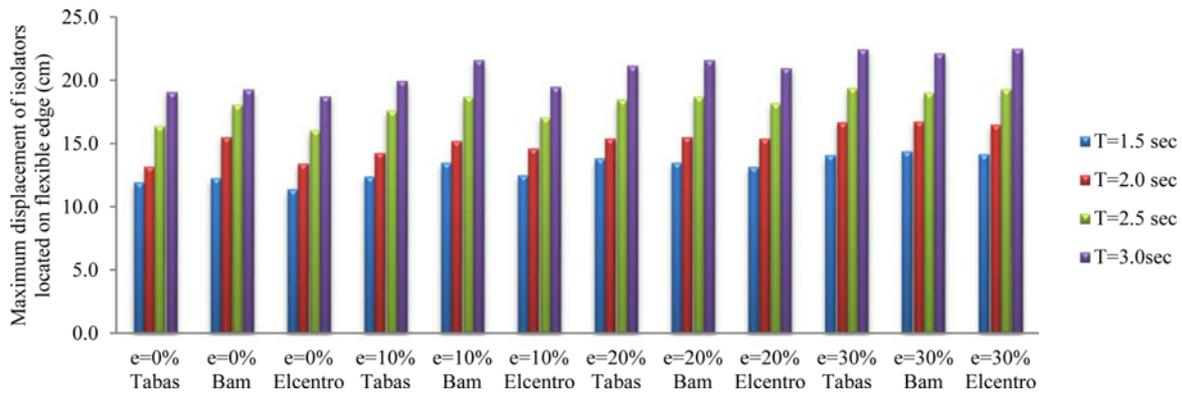
Fig. 6. Maximum Displacement of the Isolators Located on the Flexible Edge of the Isolation System with Different Eccentricities in Eight-story Structures
