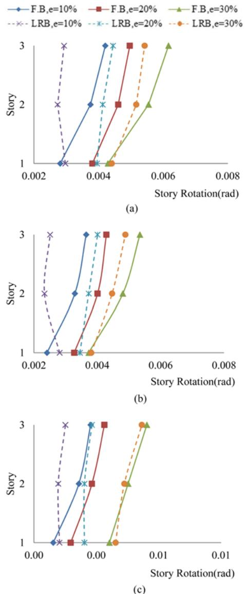
Fig. 3. Maximum Torsional Responses of the 3-Story Structure: (a) Tabas, (b) Bam, (c) El Centro
