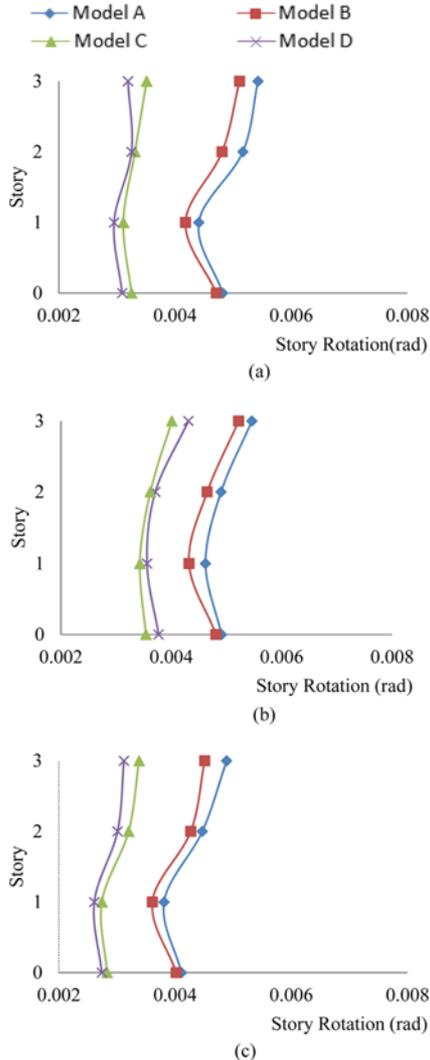
Fig. 9. Maximum Torsional Responses of the 3-Story Structural Models: (a) Tabas, (b) Bam, (c) El Centro
