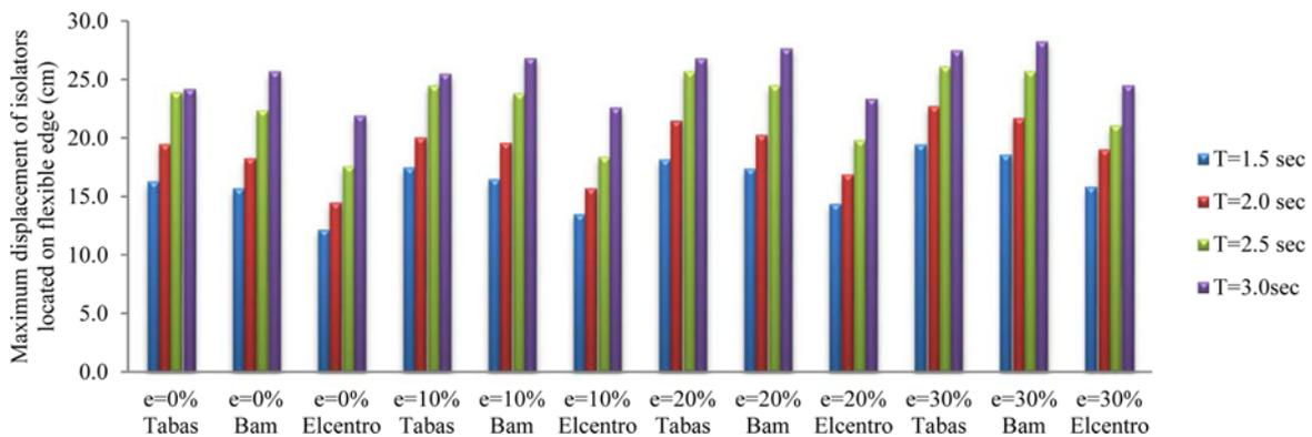
Fig. 5. Maximum Displacement of the Isolators Located on the Flexible Edge of the Isolation System with Different Eccentricities in Three-Story Structures
