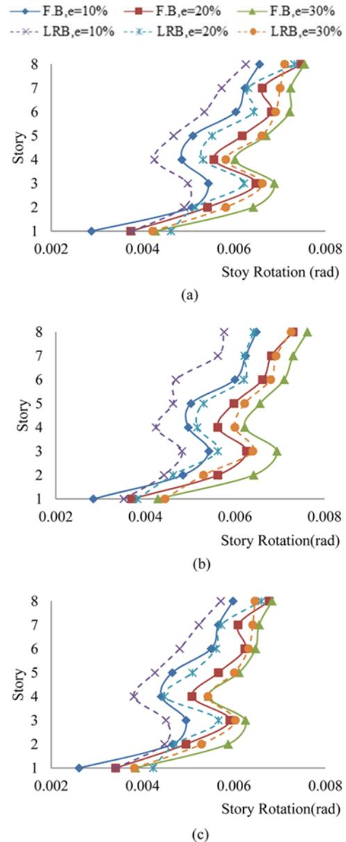
Fig. 4. Maximum Torsional Responses of the 8-Story Structure: (a) Tabas, (b) Bam, (c) El Centro
