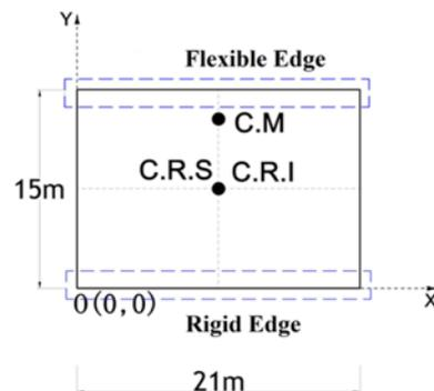
Fig. 8. C.M., C.R.I., C.R.S., Flexible Edge and Rigid Edge on the Plan of Structural Models
