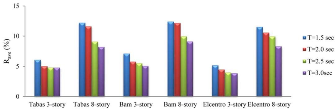
Fig. 11. Average Reduction of Torsional Responses of Model B in Comparison with Model A
