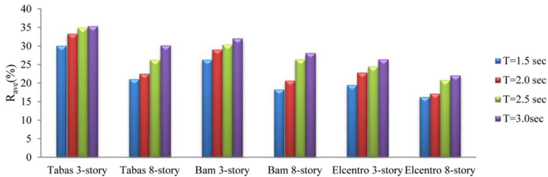
Fig. 12. Average Reduction of Torsional Responses of Model C in Comparison with Model A
