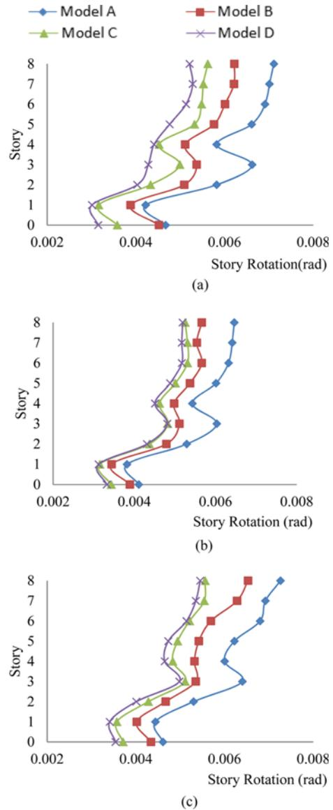
Fig. 10. Maximum Torsional Responses of the 8-Story Structural Models: (a) Tabas, (b) Bam, (c) El Centro
