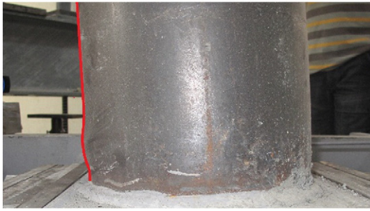
Fig. 12. Local buckling of the steel tube in a monotonic test.
