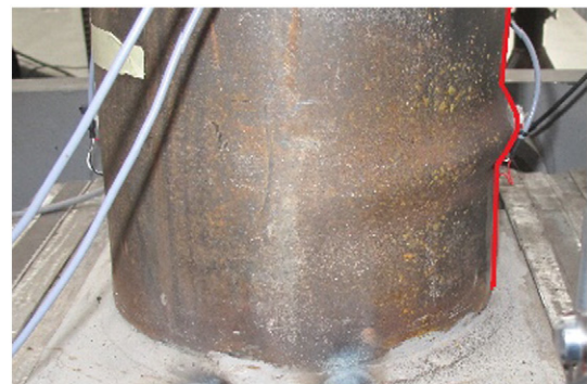
Fig. 23. Local buckling of steel specimen C219 × 3.
