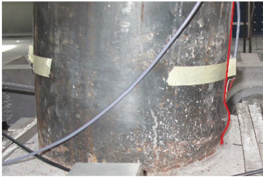
Fig. 24. Local buckling of RuCFST specimen CR-RuC15%-219-3-0%-M.
