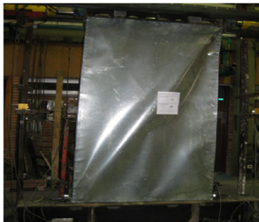
b) Tension field pattern of tested wall
