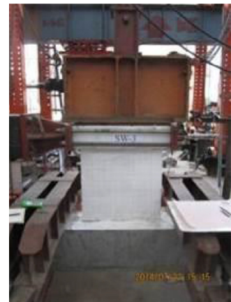
1. Wall Specimen 2. Reaction Wall 3. Hydraulic Actuator 4. Lateral Load Transfer Assembly 5. Rigidity Beam 6. Hydraulic Jack 7. Sliding Support 8. Reaction Beam 9. Rigidity Anchorage Beam 10. Rolled Screw 11. LVDTs 12. Strong Floor
