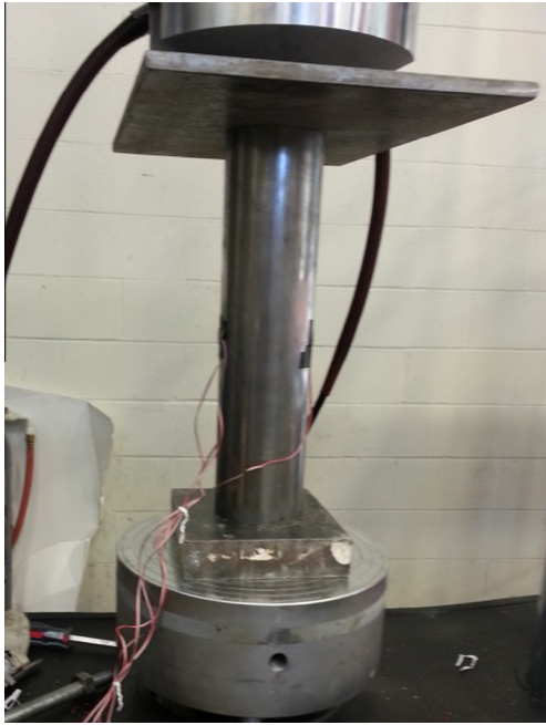
Fig. 3. Testing of steel tube under compressive loading.
