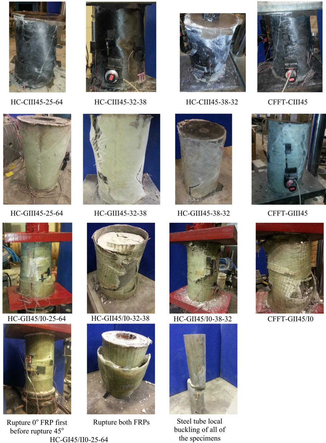
Fig. 9. Modes of failure of all of the specimens and their steel tube local buckling.
