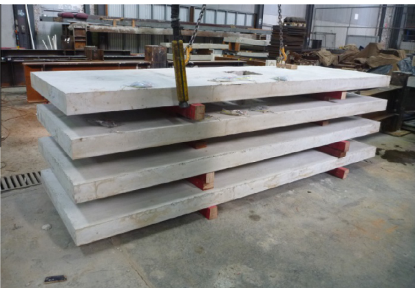
Fig. 5. Precast concrete slabs after demoulding.
