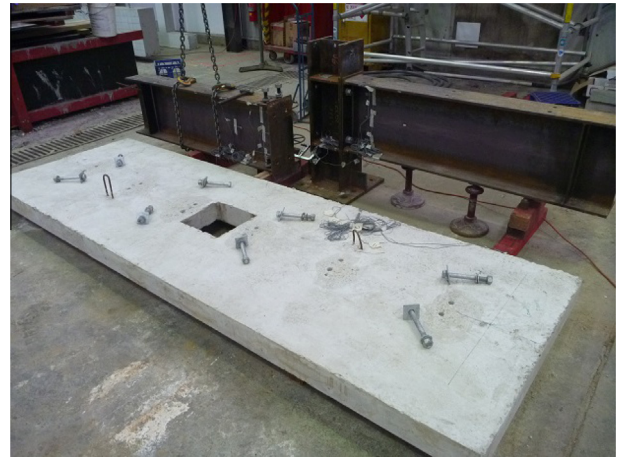
Fig. 23. Specimen CJ4 dismantled by untightening and removing the PFBSs.
