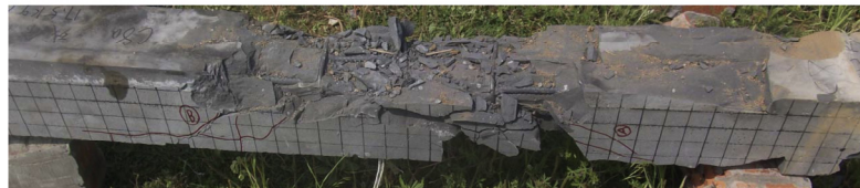
H2A Specimen with 1000 kN axial load under 17.5 kg charge weight loading
