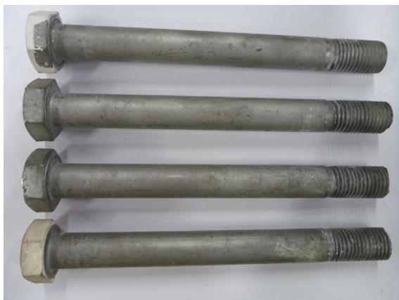
(c) bolted shear connectors after dismantling
