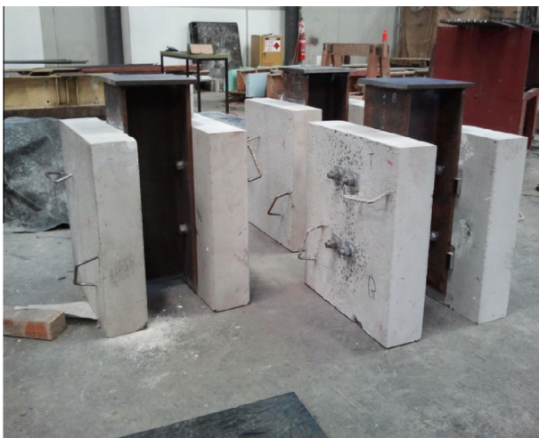
Fig. 13. Push-out test specimens.
