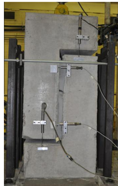
Fig. 11. Push-off test specimen after the appearance of a horizontal crack at mid-depth.
