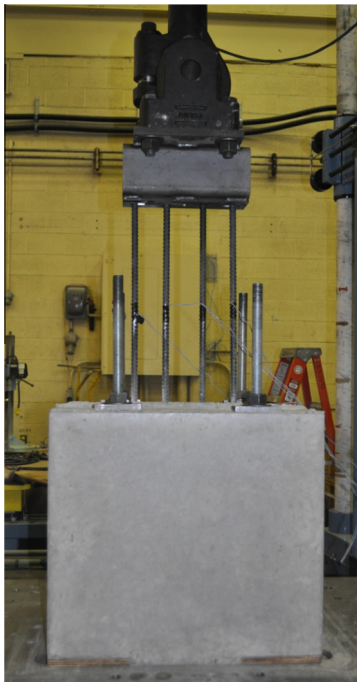
Fig. 8. Direct tension pullout test setup.
