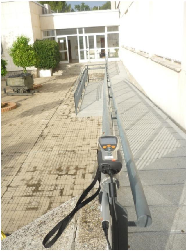
**Fig. 3.** Testo-435-4 during measurements of outdoor air in Spain.
