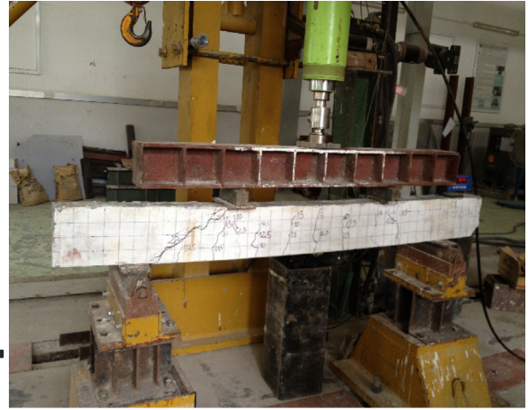
Fig. 4. Schematic of the four-point bending test.
