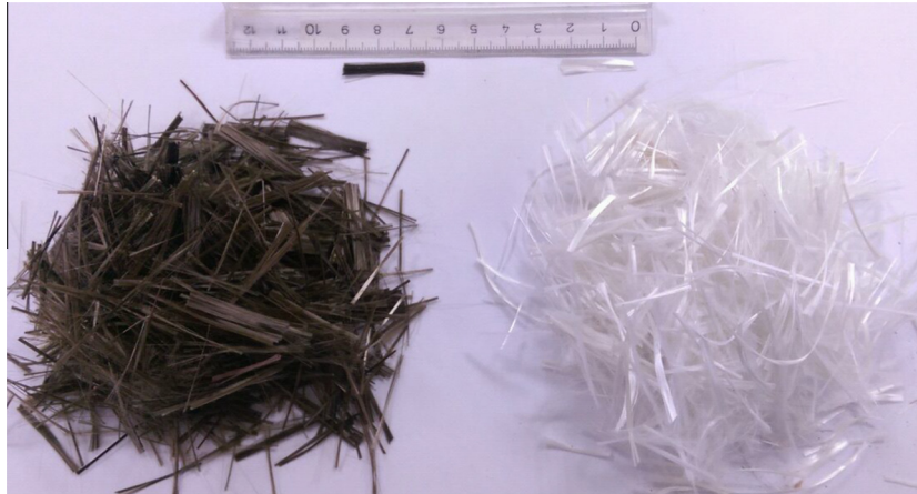
Fig. 2. Basalt and glass fibers with 24 mm length.
