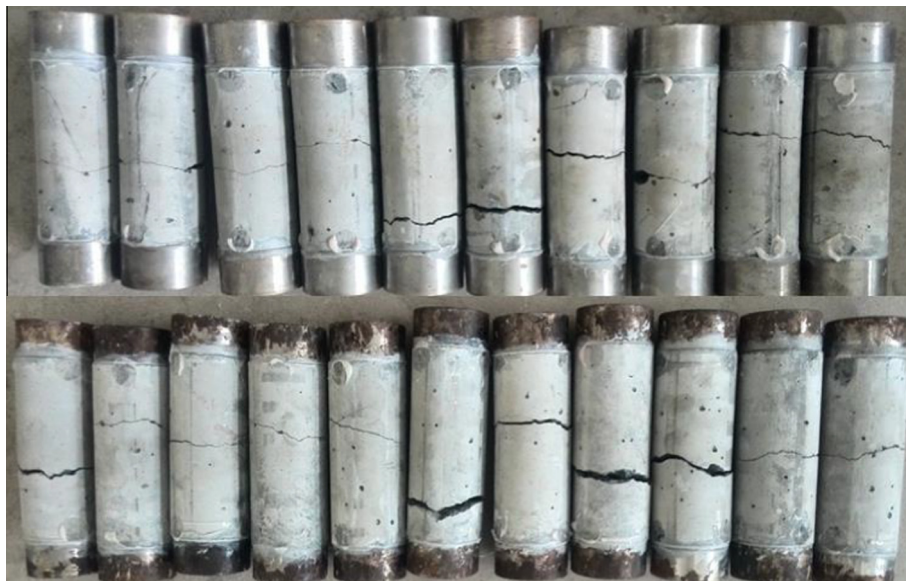
Fig. 2. The fracture pattern of concrete specimens under direct tensile loading.
