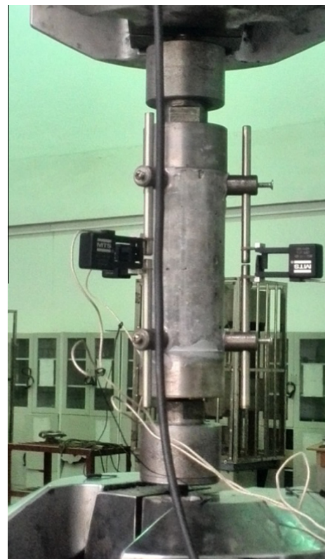
Fig. 1. Instrumented concrete cylinder.
