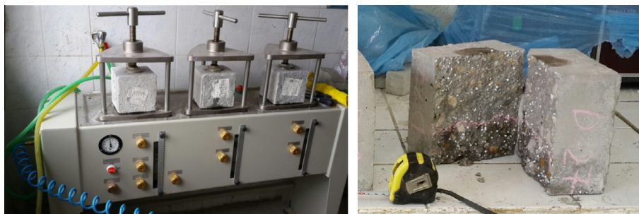
Fig. 2. Water penetration test on PCB samples.
