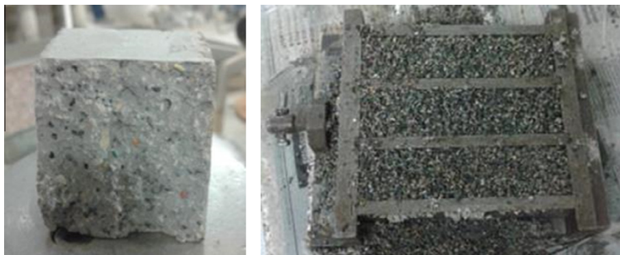
Fig. 2. On the right mortar with added plastic samples preparation by means of tooling box. On the left an image of one of the mortar samples fractured in the bending test.
