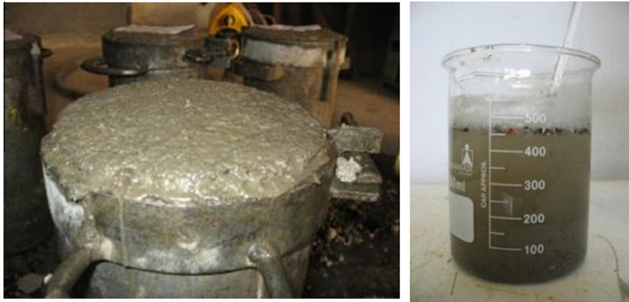
Fig. 4. Effervescence was observed during concrete samples containing PVC preparation. Sodium hydroxide solutions were prepared at different pH values and adding PVC effervescence was also observed.
