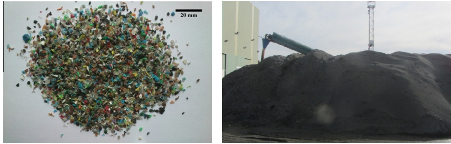
Fig. 1. On the left image showing the samples morphology coming from the recycling of electric cable sheath. On the right, image showing part of the huge amount of this kind of plastics stored in RMD (Spanish company partner of the research consortium).
