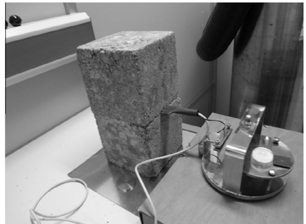
Fig. 6. Image of the concrete samples arrangement during the thermal conductivity measurements. During the experiment, the sensor is placed between two samples to be investigated, and a small constant current is supplied to the sensor, that also serves as a temperature monitor, so that its temperature increase is accurately determined through electrical resistance measurement.
