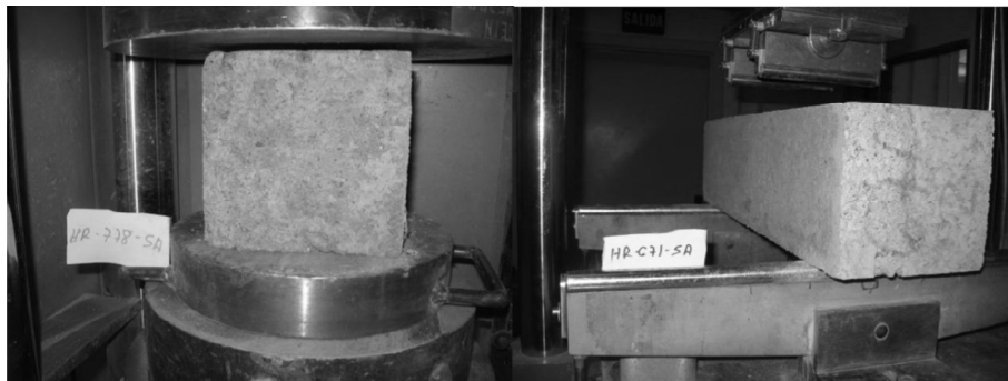
Fig. 13. On the left, concrete composite compressive test image. On the right, concrete components four point bending test.
