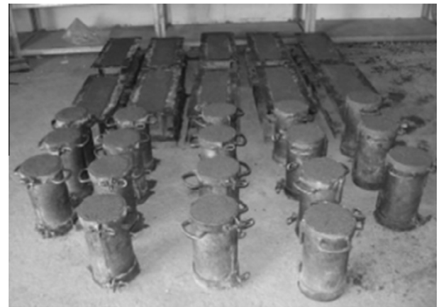
Fig. 3. Concrete samples preparation for the indirect tensile strength and bending tests.
