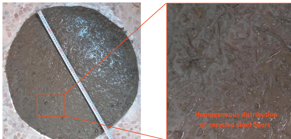
Fig. 2. The slump flow test for reinforced self-compacting concrete with 0.5% recycled steel fiber.
