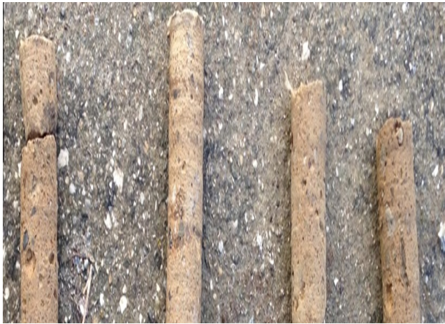
Fig. 4. Tuff samples extracted from walls for compression tests.
