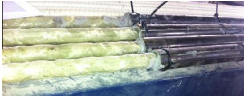
Fig. 5. Detail of the 20 mm GFRP bars used in series 2.
