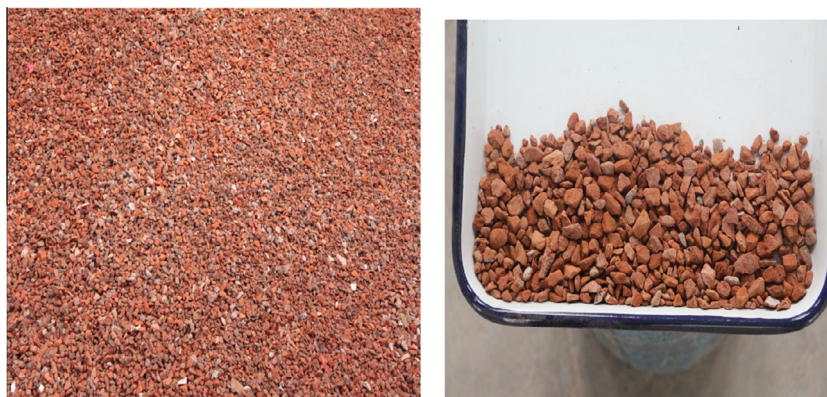
Fig. 1. The recycled clay brick aggregates ( d = 5\sim 10 mm).
