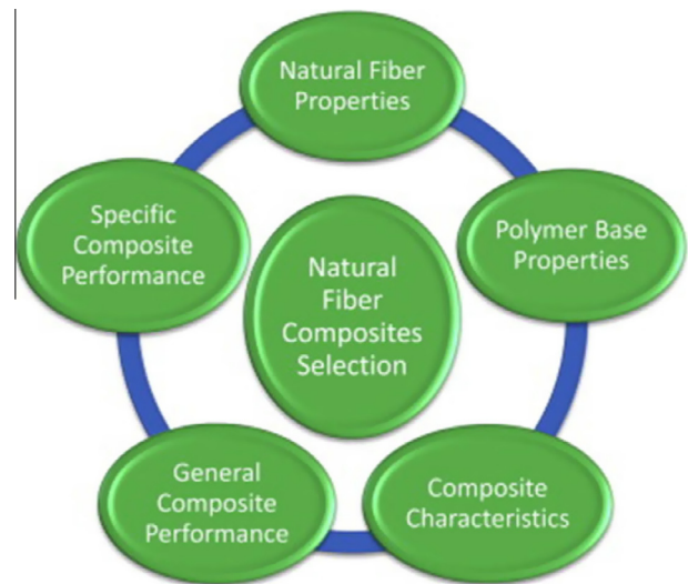
Fig. 9. Schematic diagram of criteria affecting the selection of natural fibre composite materials [59].
