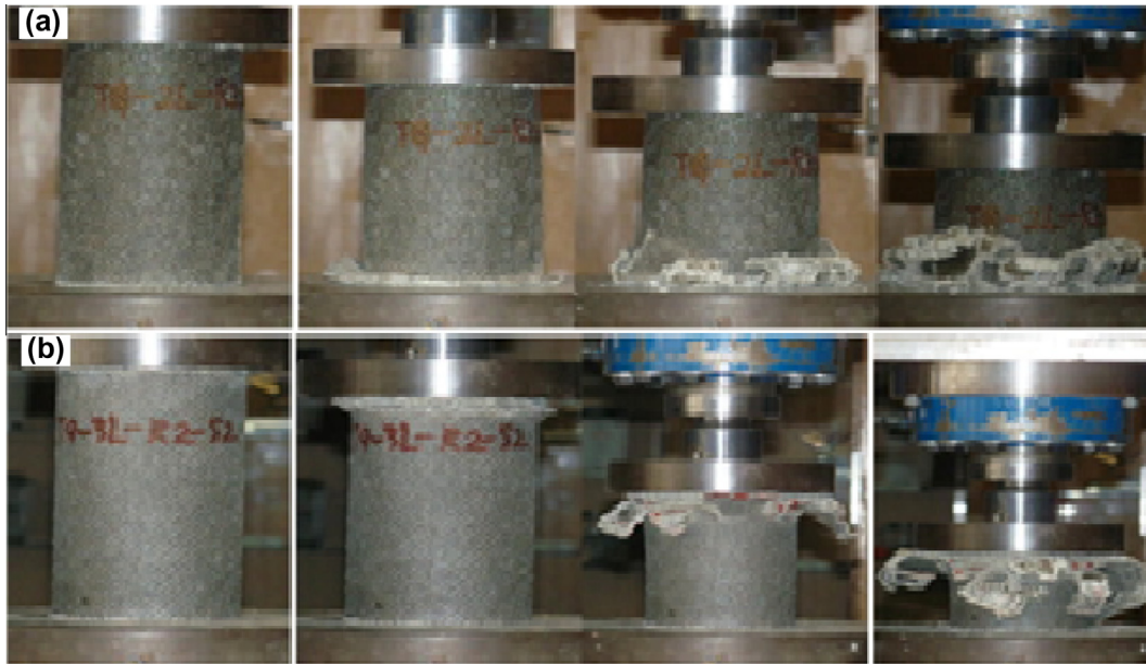
Fig. 19. Progressive crushing of specimens: (a) Mode I, (b) Mode II, [15].
